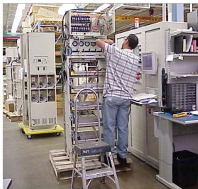
Connecting a Power Cabinet for Test
