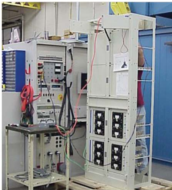
Testing a Power Cabinet in Production
